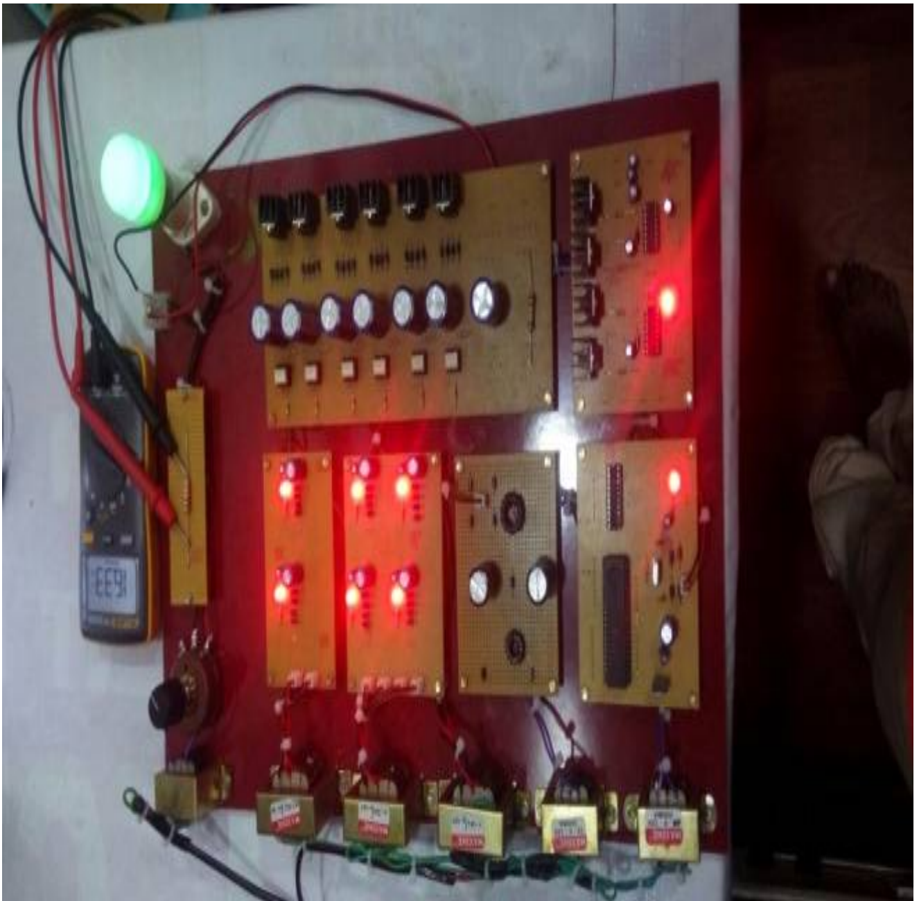
Fig:3 Hardware Snapshot Of A SINGLE PHASE 15 LEVEL INVERTER USING SINGLE DC SOURCE FOR VOLTAGE SAG COMPENSATION
